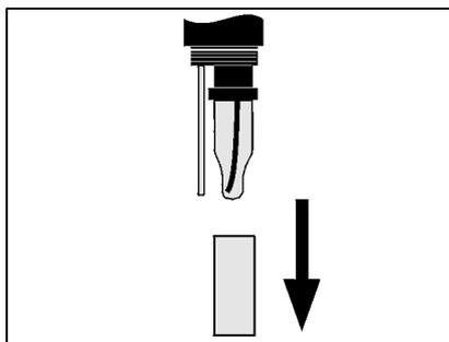
8 | Screw the protective hood onto the armature.
