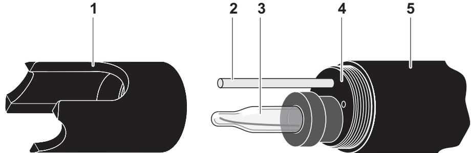
Fig. 1-1 Structure of the pH/ORP armature (example, SensoLyt® 700)
