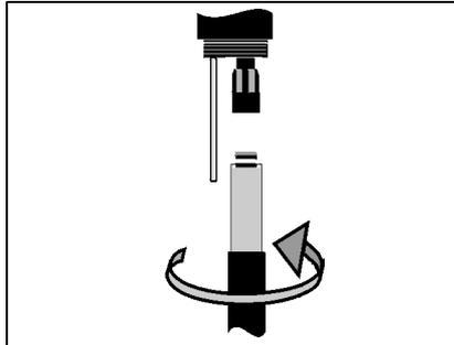
6 | Push the unit into the armature up to the stop.
